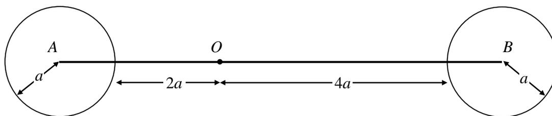
A body consists of two uniform circular discs, each of mass  $m$  and radius  $a$ , with a uniform rod. The centres of the discs are fixed to the ends  $A$  and  $B$  of the rod, which has mass  $3m$  and length  $8a$ . The discs and the rod are coplanar, as shown in Fig. 2. The body is free to rotate in a vertical plane about a smooth fixed horizontal axis. The axis is perpendicular to the plane of the discs and passes through the point  $O$  of the rod, where  $AO = 3a$ .
